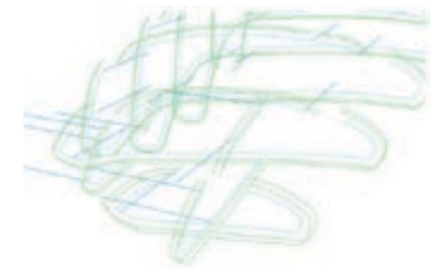
Process step 1: Input data. The basic geometry for the profiles was prepared by the engineers and handed over in a 3D CAD-file. Each profile is defined by three spline curves and a normal vector. Photo courtesy of designtoproduction
