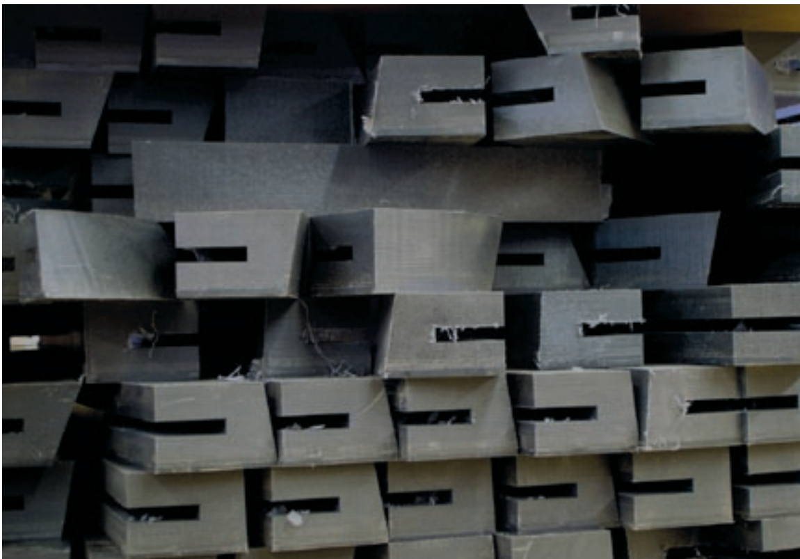
Hungerburg Funicular, Innsbruck, Austria, Zaha Hadid, 2006. Alpenzoo Station finished components stacked and ready for shipment. More than 2,500 individual such components were fabricated for the four Hungerburg stations. Photo courtesy of designtoproduction
