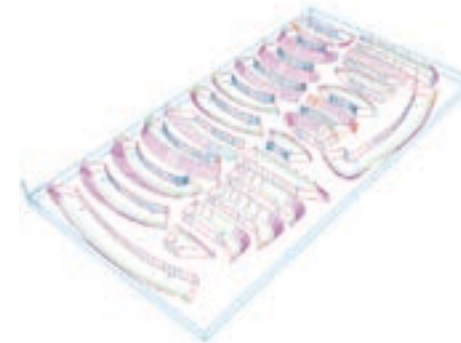
Tool positions for 5-axis cutting Every tool position is marked with a line, color coded according to the cutting angle. Photo courtesy of designtoproduction
